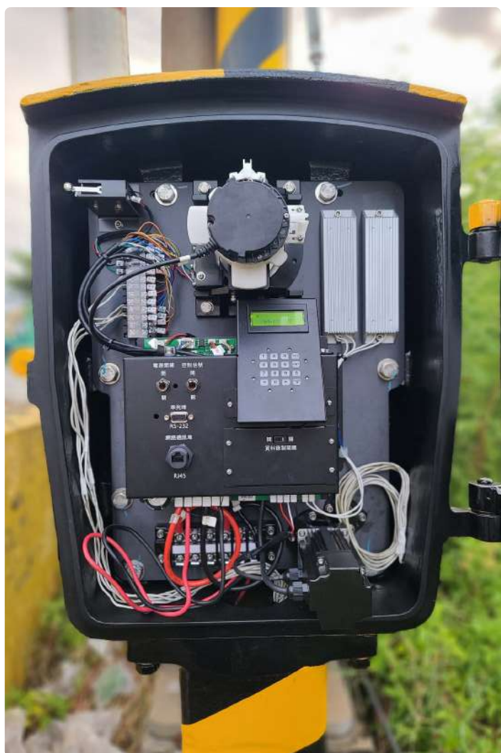
Internal Structure of the Barrier Unit
