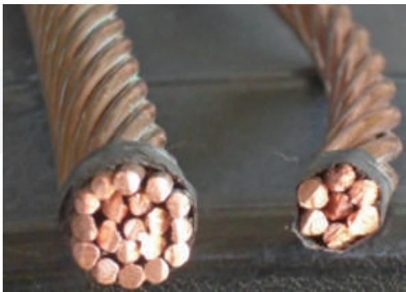
上圖為電車線主吊線(左為95mm 2 ,右為49.5mm 2 ) The picture above shows the main EMU hanging cables (the 95 mm 2 cables on the left, and the 49.5 mm 2 cables on the right.)
