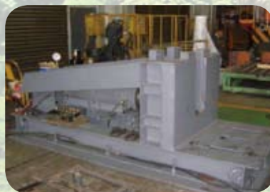
完成之車輪拆卸工作檯 Completed wheel disassembly work table
