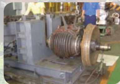
逆轉機車輪拆卸 Reversing gearbox wheel disassembly
