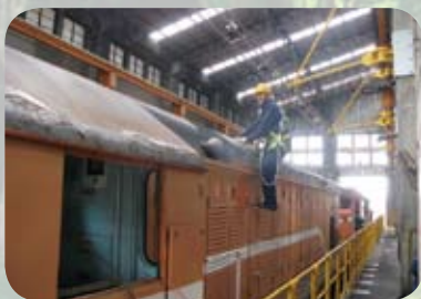
90度旋轉式車頂作業安全防護設備 90-degree Rotating Safety Equipment
