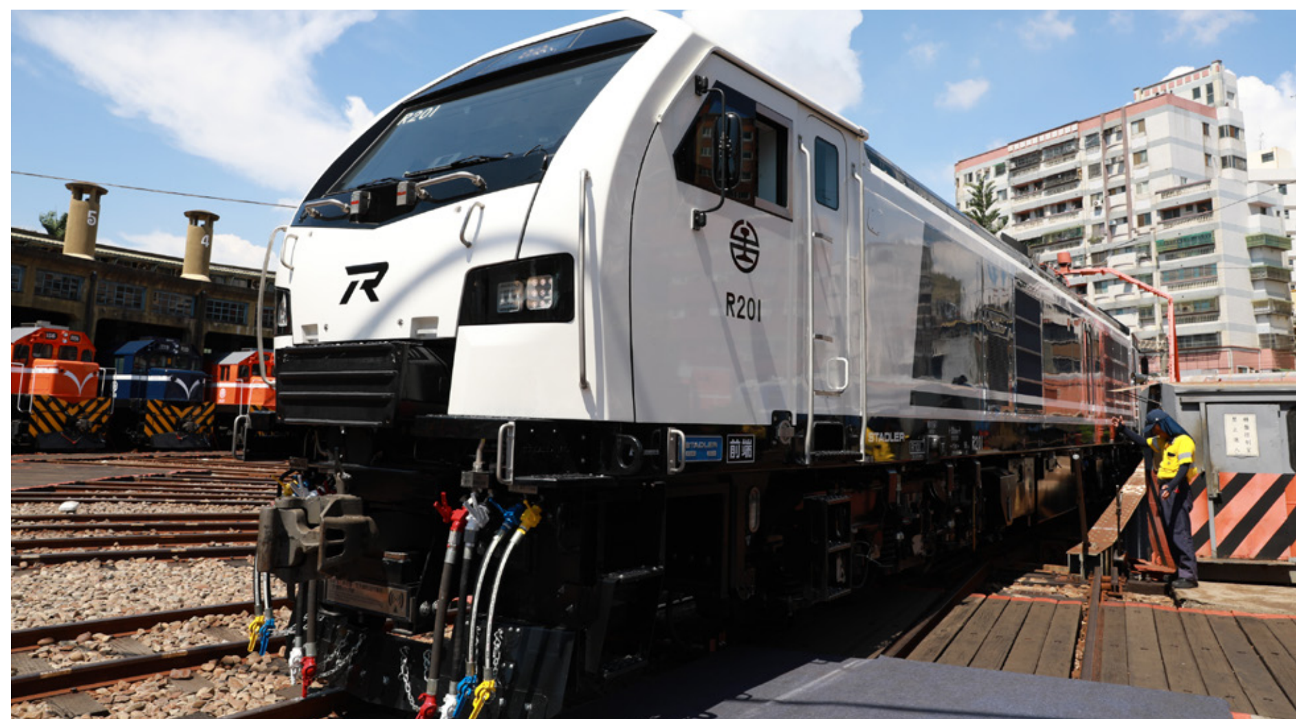
R200 new diesel-electric locomotive
