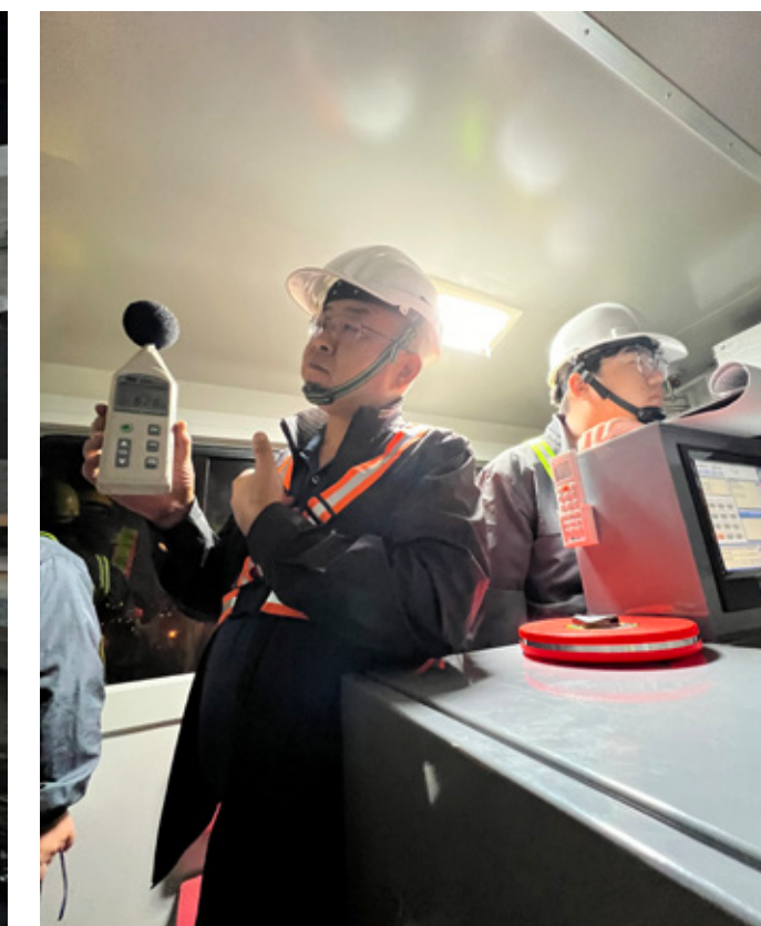
Noise test inside the boom truck
