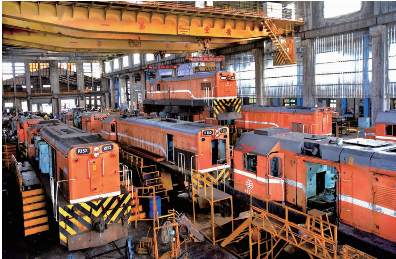
柴電工區內排滿了定期檢修的柴電機車。Trains await scheduled maintenance at the diesel power workshop.
