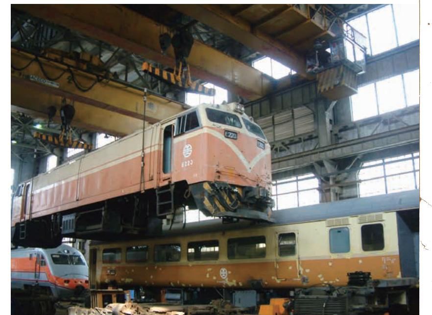
組立工場以兩部吊車同時吊掛電力機車作業 Two gantry cranes are used to simultaneously put together electric locomotives at the Erecting Shop.
