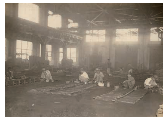
鑄鑄工場製作零件砂模鑄鑄工場製作零件砂模 At the Casting Shop, workers sand-cast parts.
