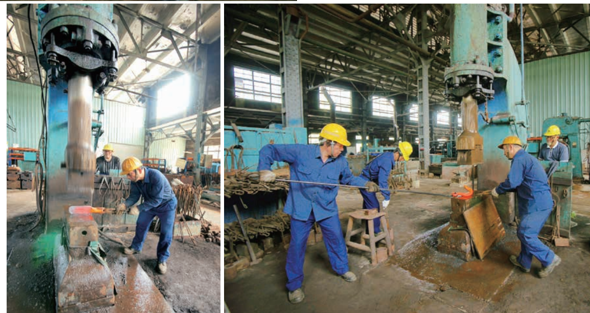
以蒸汽錘鍛造零件作業 Using the steam hammer to mold a part.
