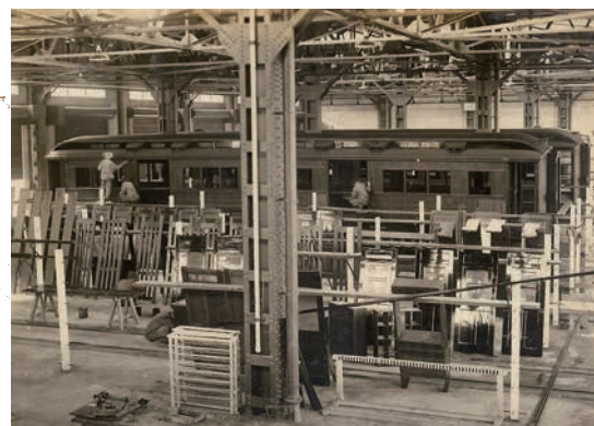
油漆工場進行車廂補土及油漆作業 Workers paint a chassis at the Paint Shop.
