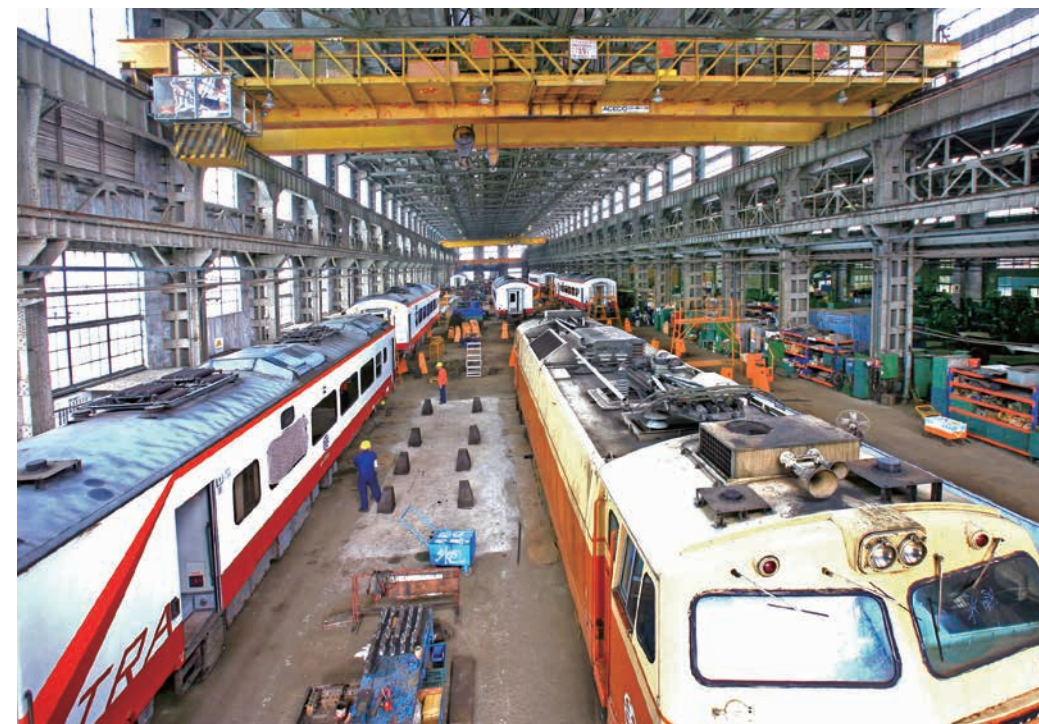
組立工場為機車最先拆卸，亦為最終組裝出場試車的工場 The Erecting Shop was where cars were assembled and disassembled.
