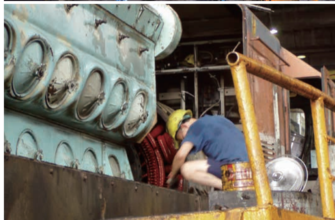
柴電機車引擎主體維修作業 A diesel engine is being repaired.
