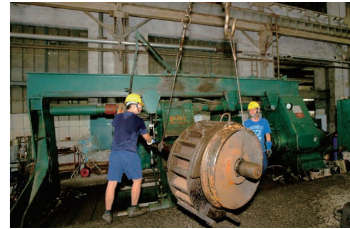
400 噸油壓機進行車輪拆卸作業 A 400-ton hydraulic press is used to remove a train's wheel.
