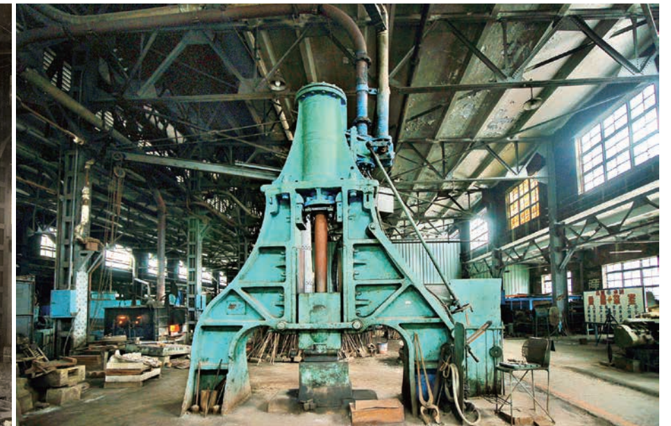
兩噸門型蒸氣錘古今對照 The two-ton door-type steam hammer, both past (left) and present.
