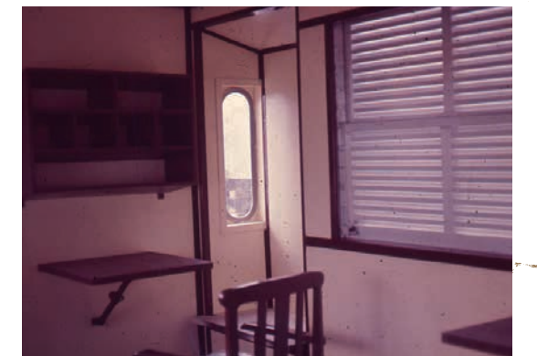
守車內可見突出的瞭望窗 Observation windows in the cabooses.
