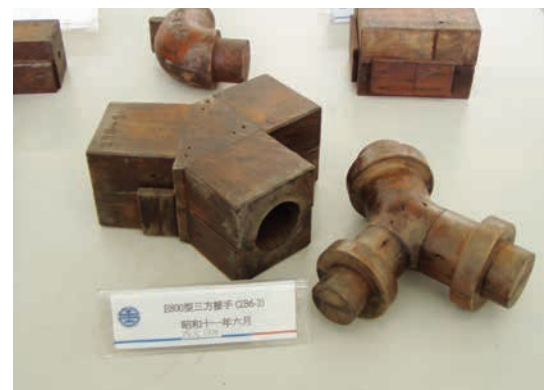
蒸汽火車接手木模 Wooden coupler molds for a steam locomotive.
