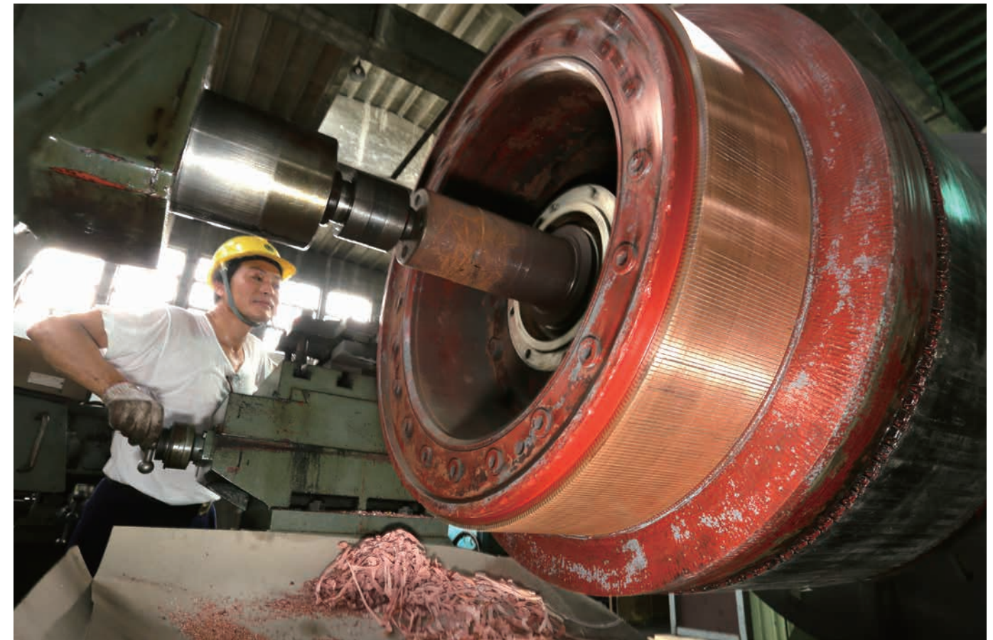
柴電機車主發電機轉子整流子面鍍削作業 A diesel-electric locomotive's dynamo is being maintained. Motor assembly at the Electric Motive Power Division.
