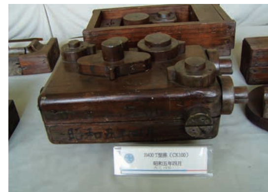
CK100 型用料木模 Wooden mold for a CK100 steam locomotive.
