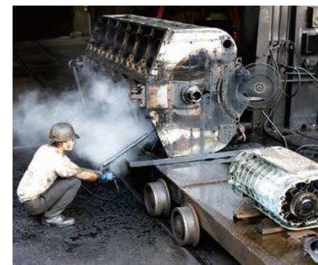
高壓熱水清洗引擎主體油污作業 Engines are steam-cleaned with pressurized hot water.
