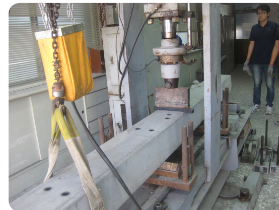
| 11. PC Sleeper Compression Test
