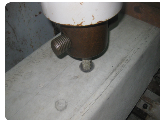
| 12. Tensile Test for PC Sleeper Bolt Hole
