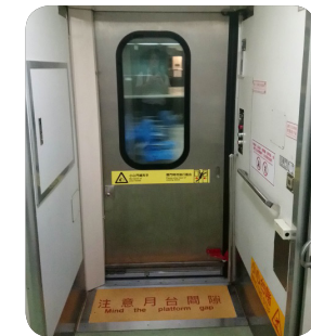
| After Removing the Stairs - Flat Ground in Front of the Door
