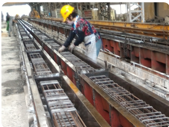
| 8. PC Sleeper Assembly Line
