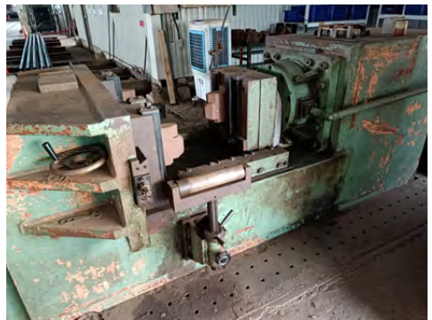
Hydraulic rail cambering machine used for bending steel rails.
