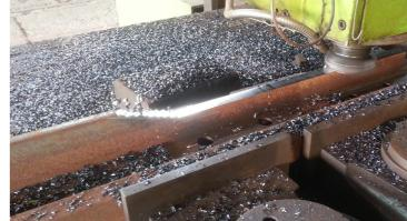
and toe of rail cutting operation
