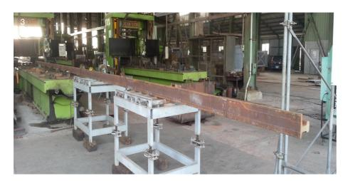
Figure 3: Use external extension support to fix the steel rail on machine
