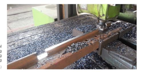
Figure 9: The step side cutting is completed Step side cutting
