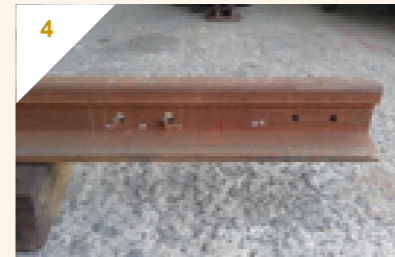
4 Mark the processing area on the rail web
