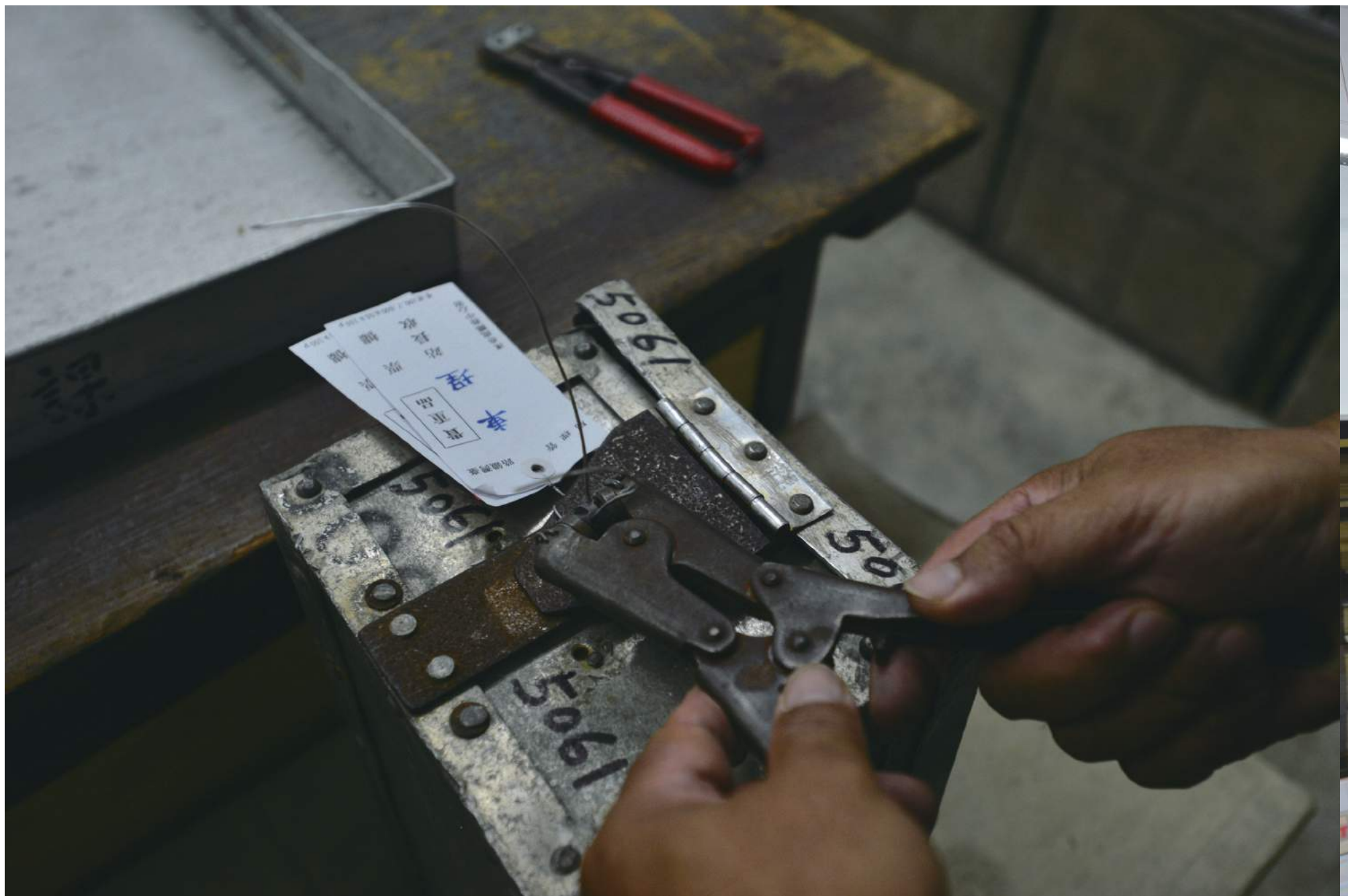
裝箱完成後進行鉛封 The lead-sealed box loaded with tickets.
