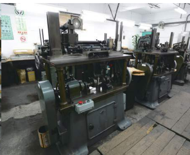
日本國友鐵工所製的硬票印製機 Ticket printing machine made by Kunitomo Co. in Japan.
