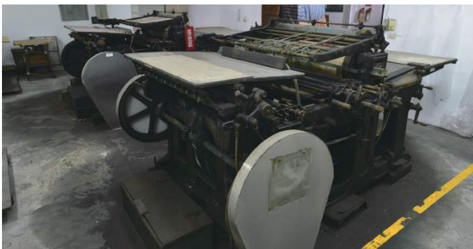
底紋活版印刷機 Typography press for printing cardboards.
