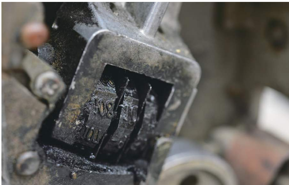
天虎牌軋日機的日期字盤 The number types of the Tenko dating machine.
