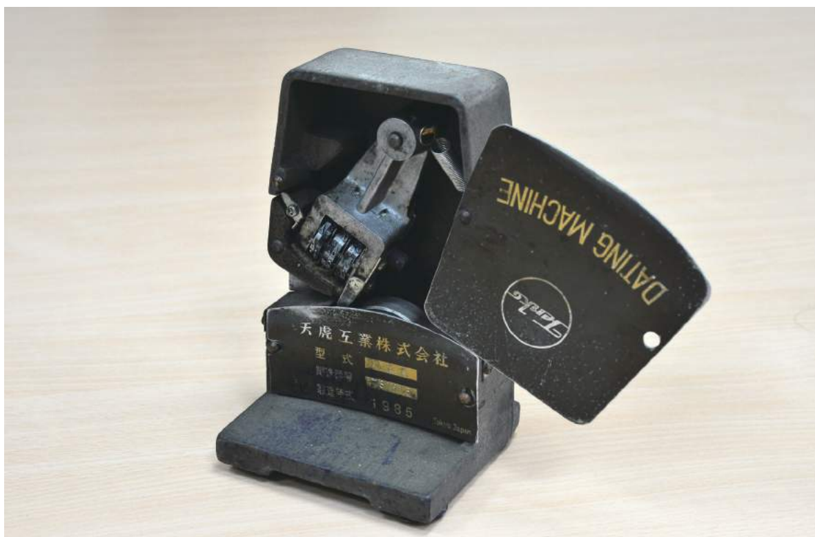
天虎牌軋日機的內部構造 The inner structure of the Tenko Dating Machine.
