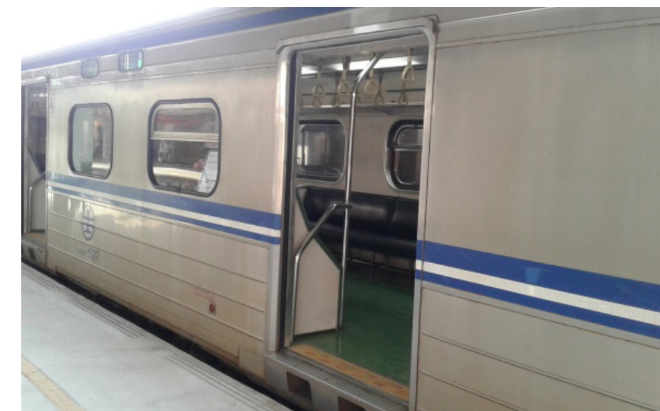
Entrance is flush with the platform after stairless construction
