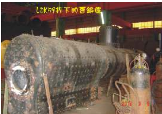
LDK59拆下之舊鍋爐
