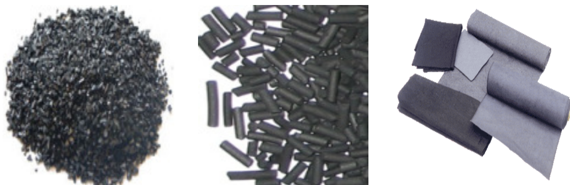
(a) G840顆粒狀圓柱碳 (b) G306圓柱狀圓柱碳 (c) AM1132活性碳纖維氈 圖5活性碳型態
